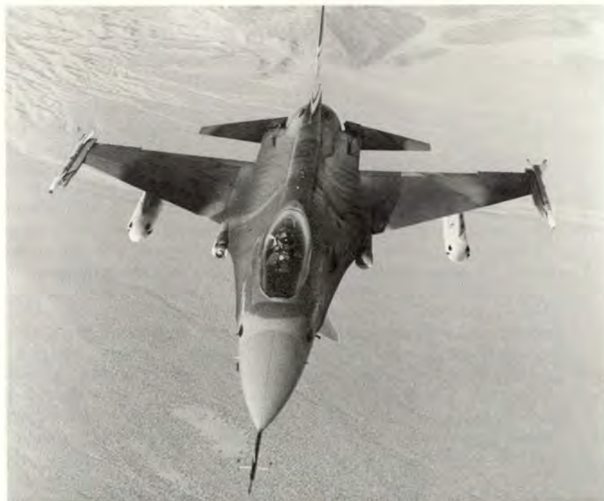
Figure 1. The GCAS computer constantly calculates altitude needed to recover above the MDA. The system begins warning the pilot visually and aurally 5 seconds before taking control. If the pilot doesn't respond, the GCAS will perform a flyup maneuver at the last second.
